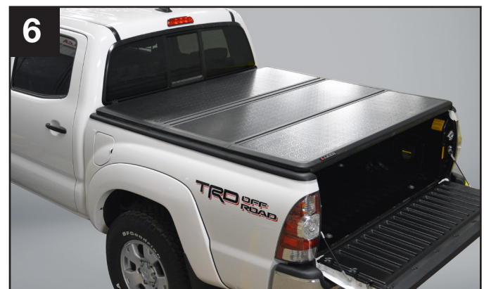
6.) With tailgate open and front cab latches secure, unfold cover completely.
