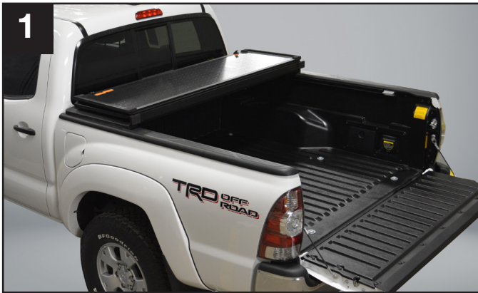
1.) Wash truck bed. Place the cover on front of truck bed (cab end).
