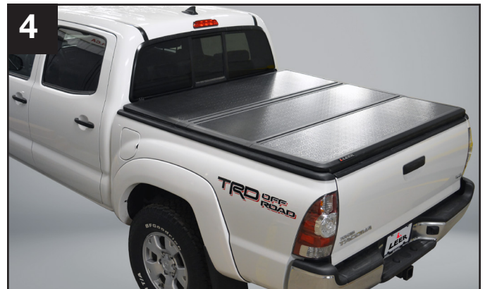
4.) With tailgate closed, unfold cover fully. Adjust position over the truck bed for proper cab/tail alignment before securing latches.
