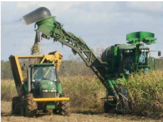
No matter what type of crop or field, Donaldson TopSpin pre-cleaner stops debris and chaff from entering the intake during harvesting to extend the life of the primary filter.
