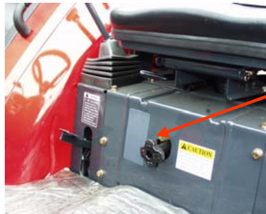
Adjust knob of hydraulic descent speed
