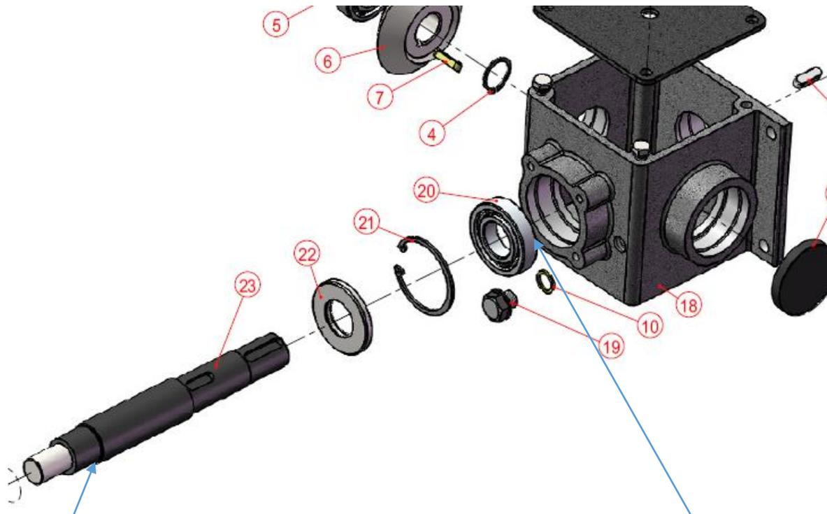
Installed a 1.5" internal snap ring behind bearing # 20 inside the gearbox
