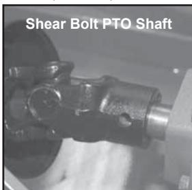
Shear Bolt PTO Shaft
