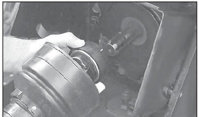
7. Support and collapse driveline completely and lower onto PTO holder.
