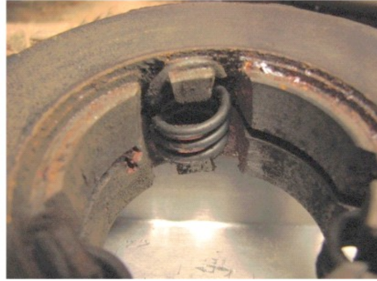
Note the heavy springs holding the plates together.
