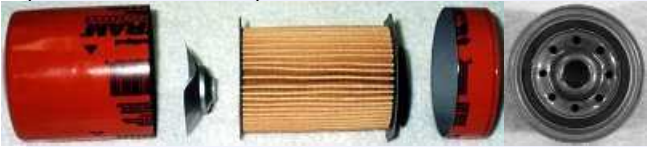
Exploded view and backplate:
