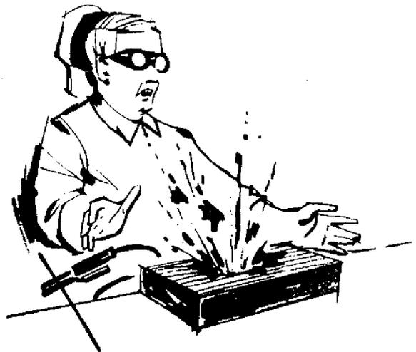
Figure 1-6. Don't weld on hollow (cored) castings
