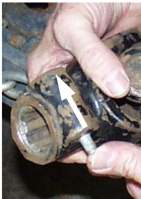
Figure 5.4.e. The push pin detent lock on the PTO driveline has a metal rod which fits in the PTO stub shaft groove to secure it. A firm grip is needed to press the pin. Do you have enough hand strength to push this pin in all the way?
