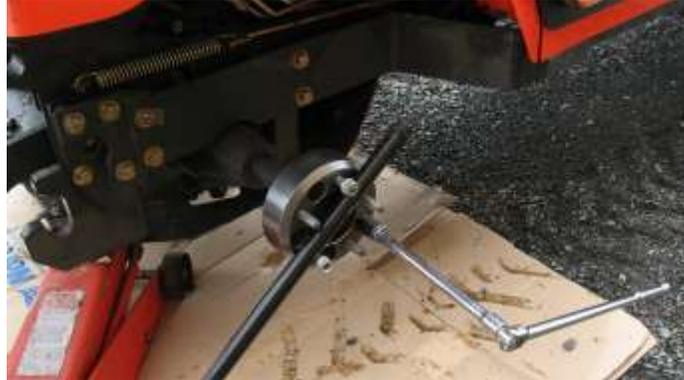
H. Get your Tire/Rim & add Loctite to the 6 studs on the spacer. You will need to use the supplied nuts & reuse the 2 factory nuts & all the Washer/lockwasher to install the rim/wheel. Torque the nuts to 140 ft. lbs for the rear wheels in the same 3 steps as above.
