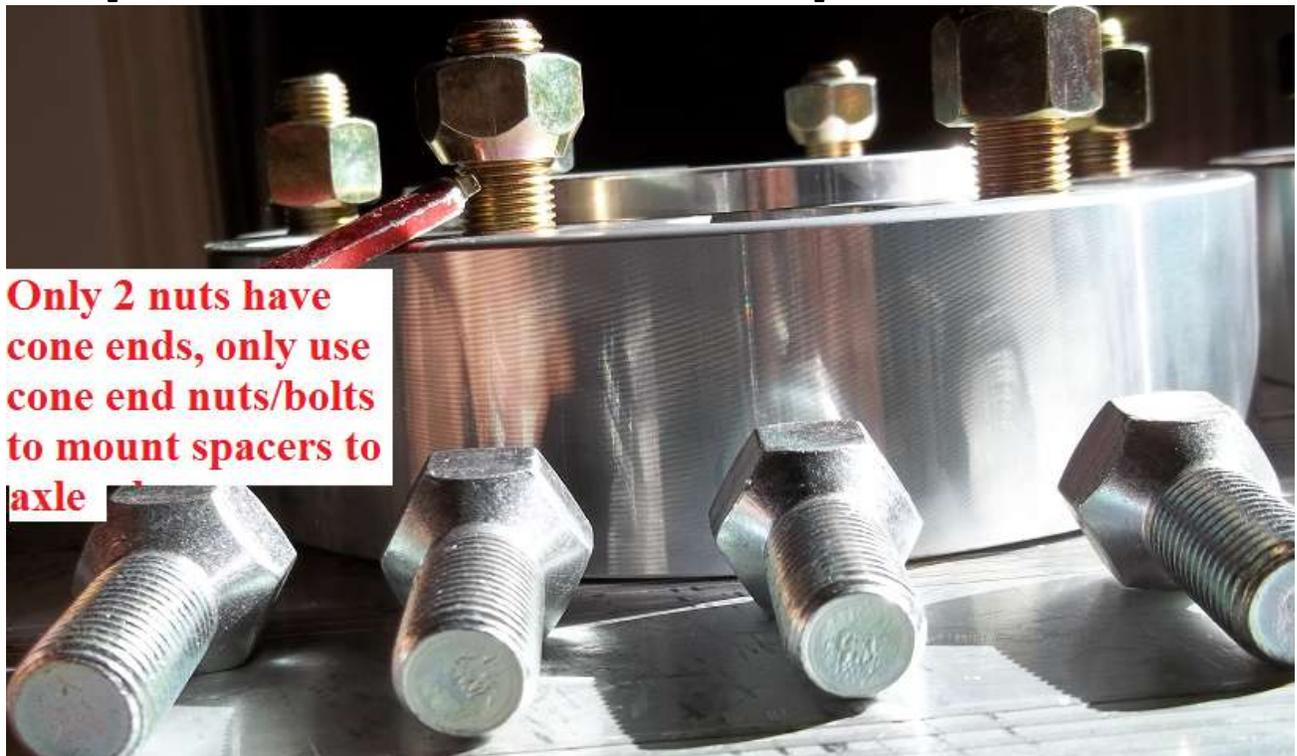
⚠ Please take the time to make the install in a 3 steps. First hand tighten the bolts; Second torque the bolts to half the torque in a crisscross pattern & Finally torque the bolt to their final value of 140 ft. lbs for the rears wheels.
