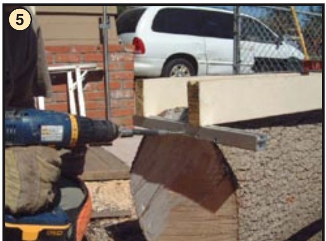
Attach brackets to one end of the log. You may need to drill and toe nail the 2 x 4 to stabilize the guide on the other end.
