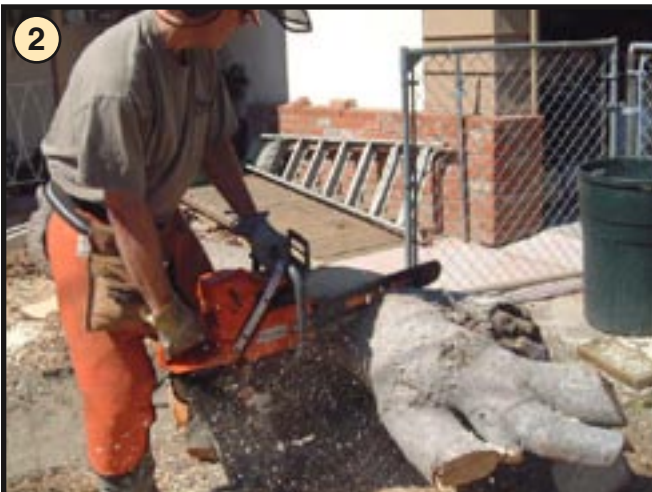
Trim the log to the length necessary to fit your first cut guide system.
