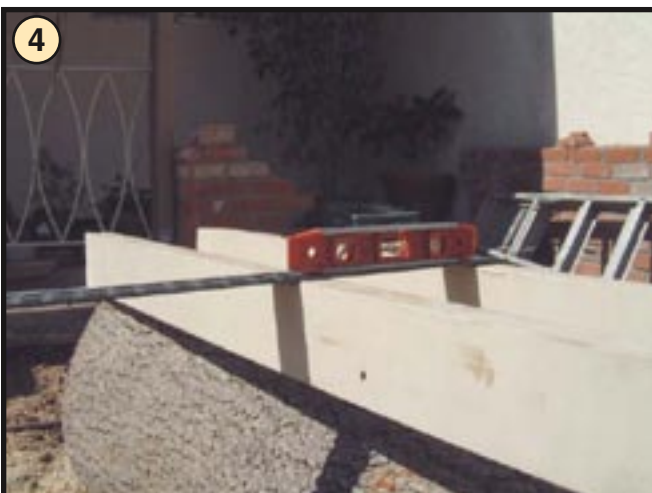
Level guide system in cross direction. If the log tapers from one end to the other and you want to cut down the center of the log, then you may need to raise one end of the guide system up.
