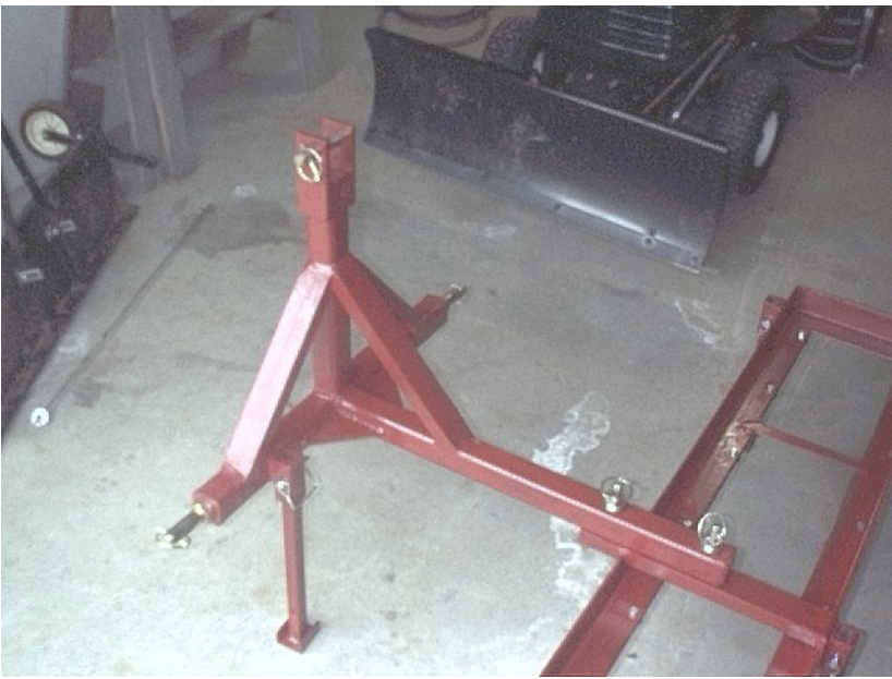
Close-up of general purpose hitch. Notice diagonal C channel supports and drawbar parking stand.
