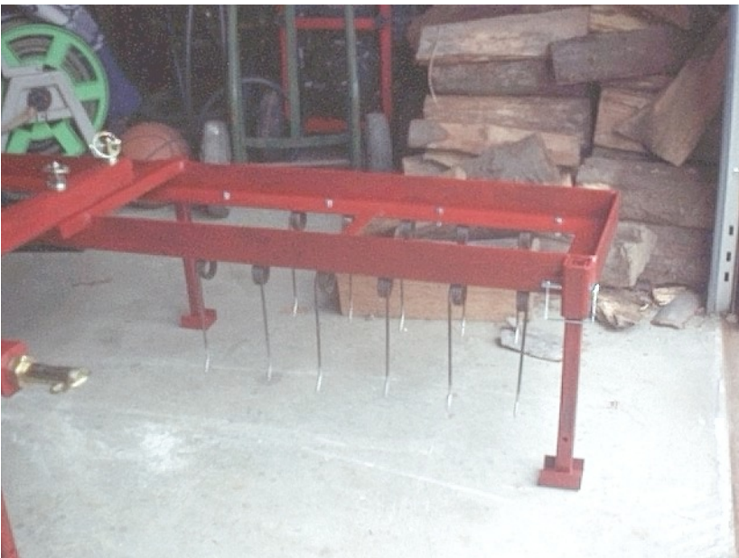
View of tine alignment and front left parking stand. Front right parking stand will be located between the first 2 tines (see above photo).
