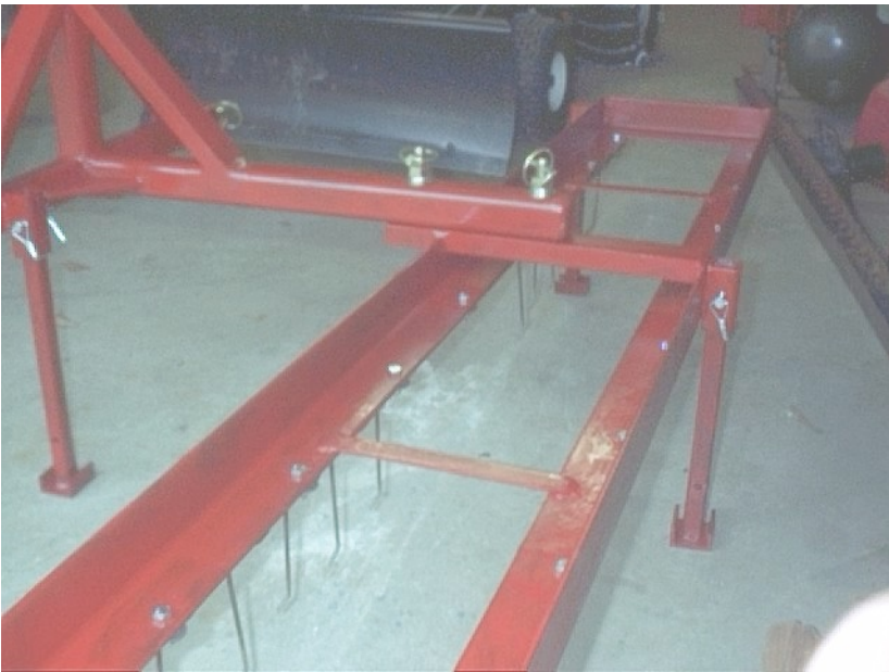
Close-up of hitch arm connection and rear parking stand. Notice how hitch mount is connected on the left by notching the C channel "ears". Also shows optional supports installed.
