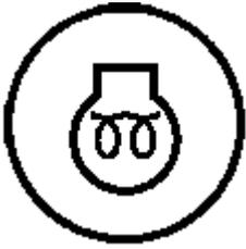
**(4) Preheat Light** - The indicator comes on when the engine start switch key is turned to the ON position. The glow plug will preheat at this time to aid in cold weather starting. The indicator goes off after the engine is started.
