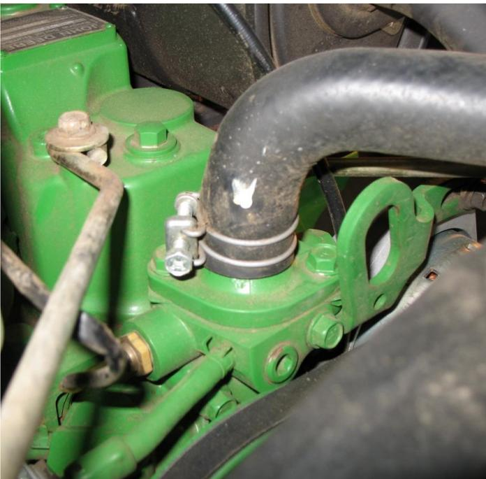
**Note:** The HOSE CLAMP (IPL KEY # 2) Assembly has a combination Phillips Hex Head Bolt. Due to space constraints I have called for a RATCHET WRENCH.
