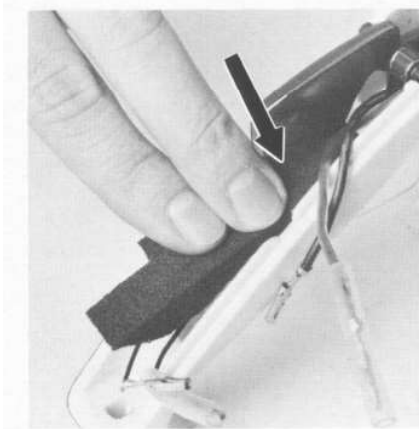
Fitting pressure pad
